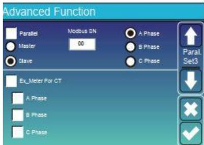
**Ex\_Meter For CT:** when in Three phase system with CHNT Three phase energy meter (DTSU666), click corresponding phase where hybrid inverter is connected. e.g. when the hybrid inverter output connects to A phase, please click A Phase.
