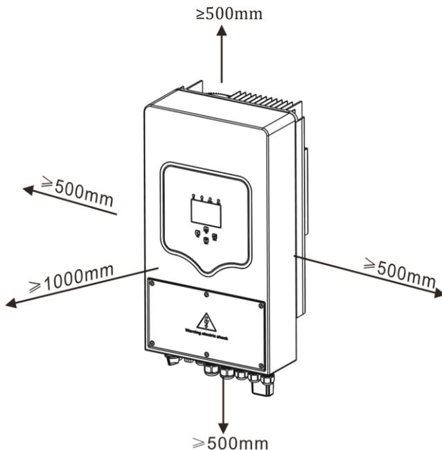
For proper air circulation to dissipate heat, allow a clearance of approximate 50cm to the side and approximate 50cm above and below the unit. And 100cm to the front.
