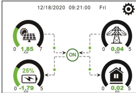
1. The icon in the center of the home screen indicates that the system is in the 'Normal operation' mode. If it turns into "comm./FXX", it means the smart inverter has communication error or other errors, the error message will display under this icon (FXX errors, detail error info can be viewed in the System Alarms menu).
