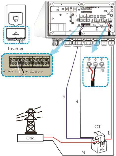
**\*Note: when the reading of the load power on the LCD is not correct, please reverse the CT arrow.**
