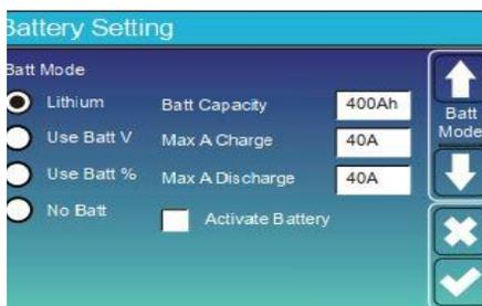
**Battery capacity:** it tells JSO smart hybrid smart inverter to know your battery bank size.
